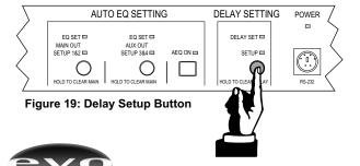
Pressing any button during the Delay Setting routine will abort the process and settings will return to previous values.
